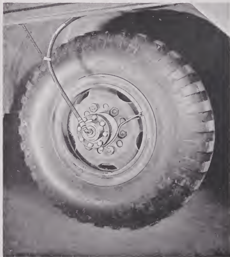
FIGURE 26. Early proposed hub arrangement for central tire-inflation control.
